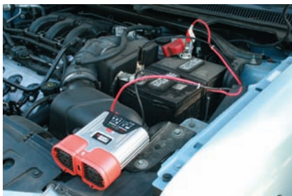
For 500W power connect to the battery with clamps.
